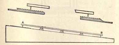
a flat bar of an expansible metal, provided with equidistant rows of teeth along its upper and lower ends, and made to rest on an inclined slab of slightly expansible material, in which horizontal grooves are cut as close to one another as possible.
